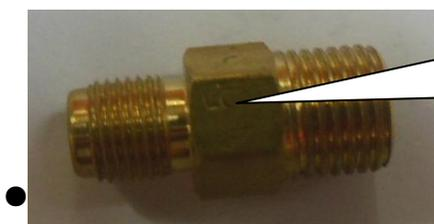
Injector of Pilot Burner.
